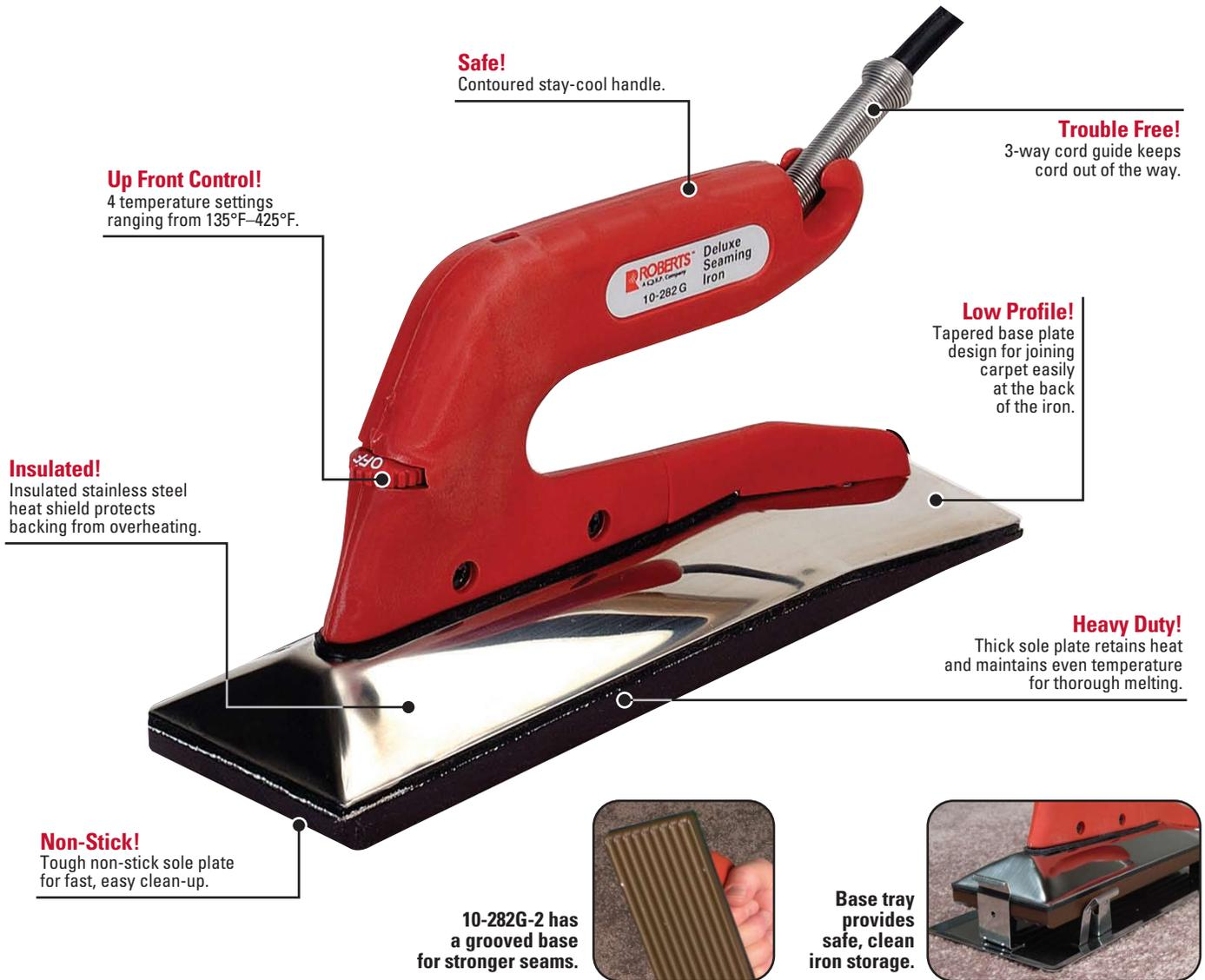
*These Roberts Deluxe Carpet Seaming Irons have an adjustable thermostat and heat shield to provide ideal heat for hot melt tape while protecting carpets from high temperatures. Streamlined, low profile design provides even heat distribution for thorough melting and easy carpet seaming. These irons have a heat range of 135°F to 425°F.*
